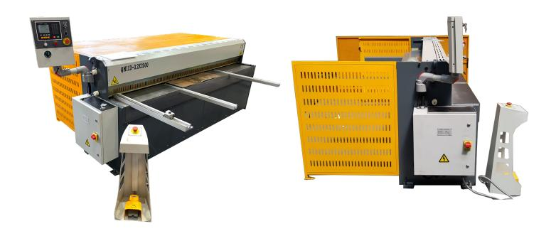
Our range of mechanical & hydraulic guillotines have been in development for many years. With 2 ranges, mechanical and hydraulic we have all your bases covered when it comes to sheet metal cutting. **Mechanical Guillotines** can process **up-to 3.2 mm** in thickness (whereas our premium **Hydraulic Guillotines** can process **up-to 20mm** in thickness).
